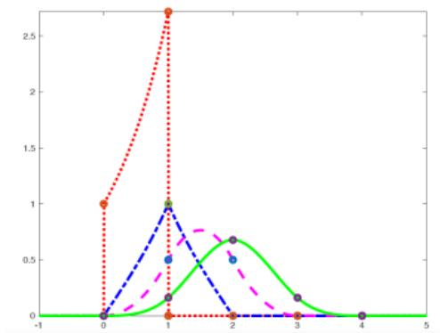
Cardinal HB-splines of order 4 (green) is obtained by convolution of 4 HB-splines of order 1 (red)
