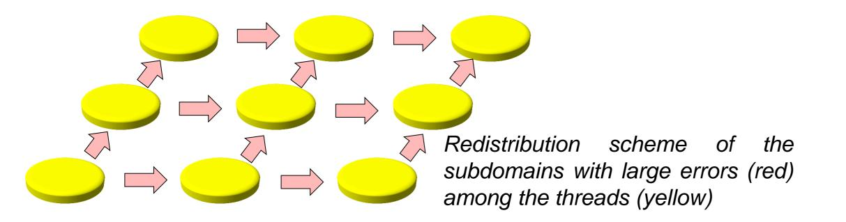
the function evaluations  $f(x_i)$  in the basic rule r are independent and can be executed by different threads of the GPU
